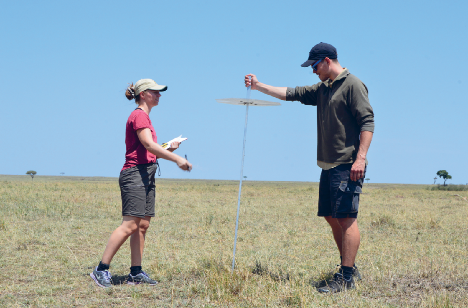
Figure 3. BIOCHANGE students are using a drop disc to estimate the grass biomass in the Mara North Conservancy, Maasai Mara, Kenya. Photo: Louise V. Sørensen, BIOCHANGE.
