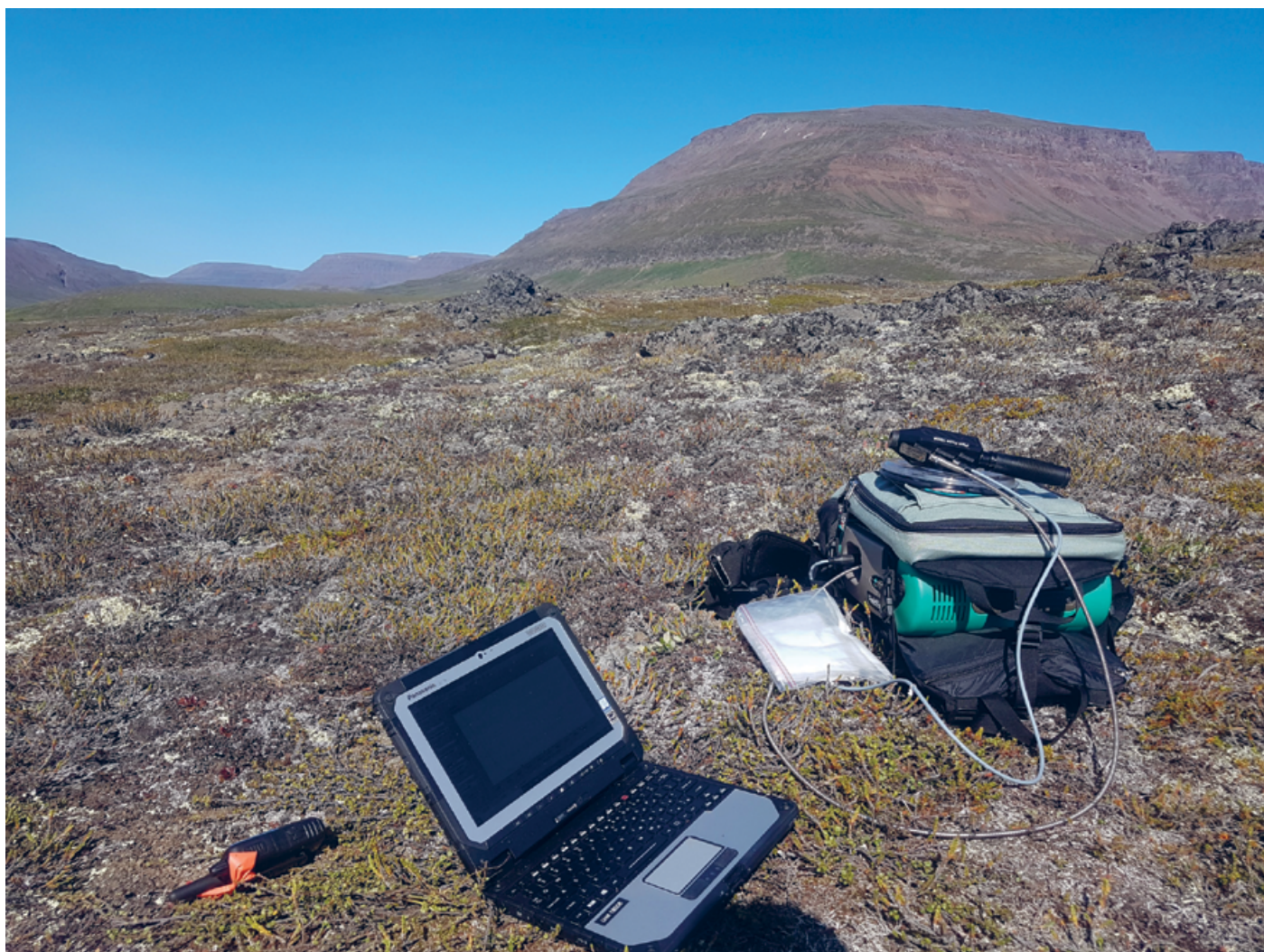
Figure 4. How does spectral bio- and geodiversity relate? Field spectrometer used to measure spectral analyses of leaf and soil samples at Disko Island, Greenland. Photo: Oliver Baines.
