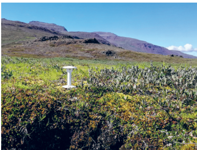
Figure 3. TMS logger installed in each plot measuring temperature in different strata above- and belowground as well as soil moisture. Photo: Urs A. Treier, BIOCHANGE.
