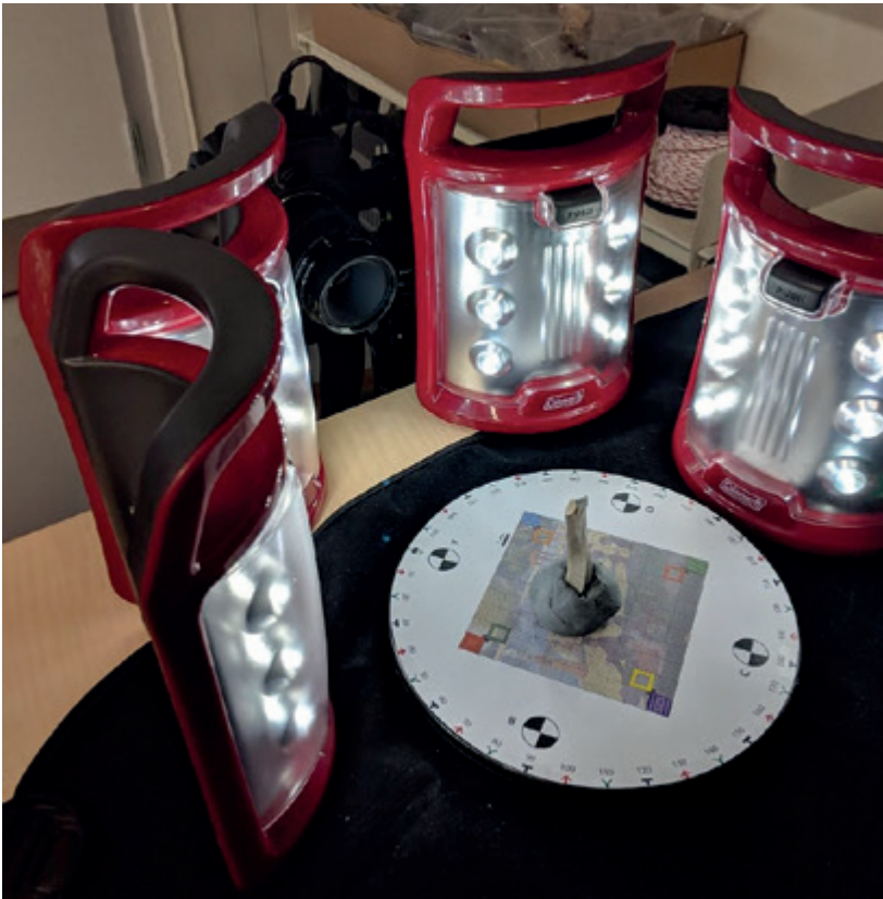
Figure 1. The structure-from-motion set-up (Camera: 50MP Canon EOS Full Format). Photo: Christian Steven Hoggard, BIOCHANGE
